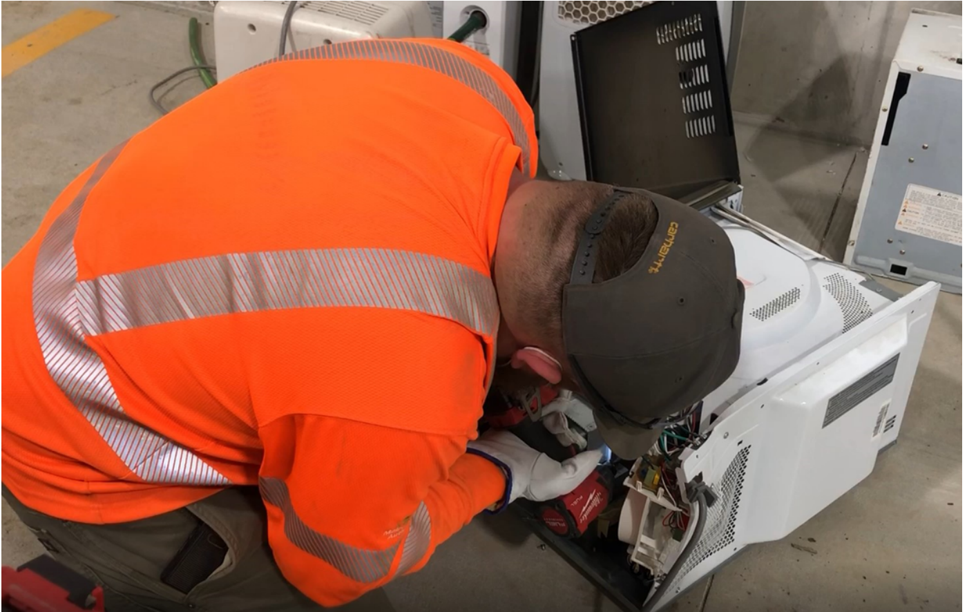
This photo shows a staff member demanufacturing an appliance.
